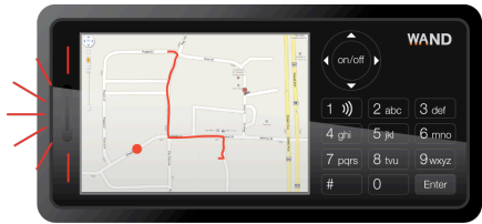
figure 3: Using GPRS the device can detect and alert the caretaker when their child is off their path.
