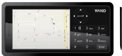
figure 1: Prototyped WAND device with stylus and map of home area.
